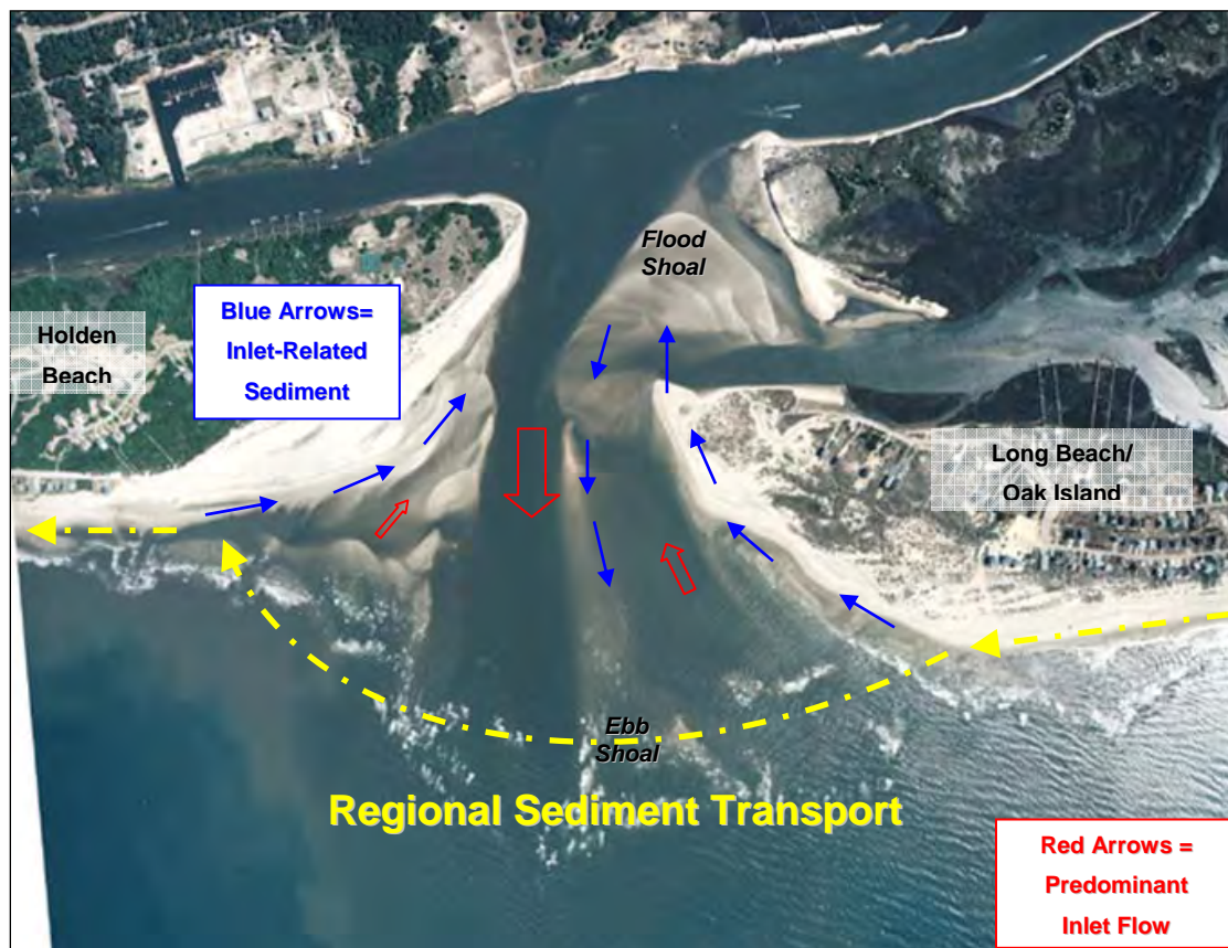
Figure 5-1: Conceptual regional and local net sediment transport schematic at Lockwoods Folly Inlet (2004 aerial).
