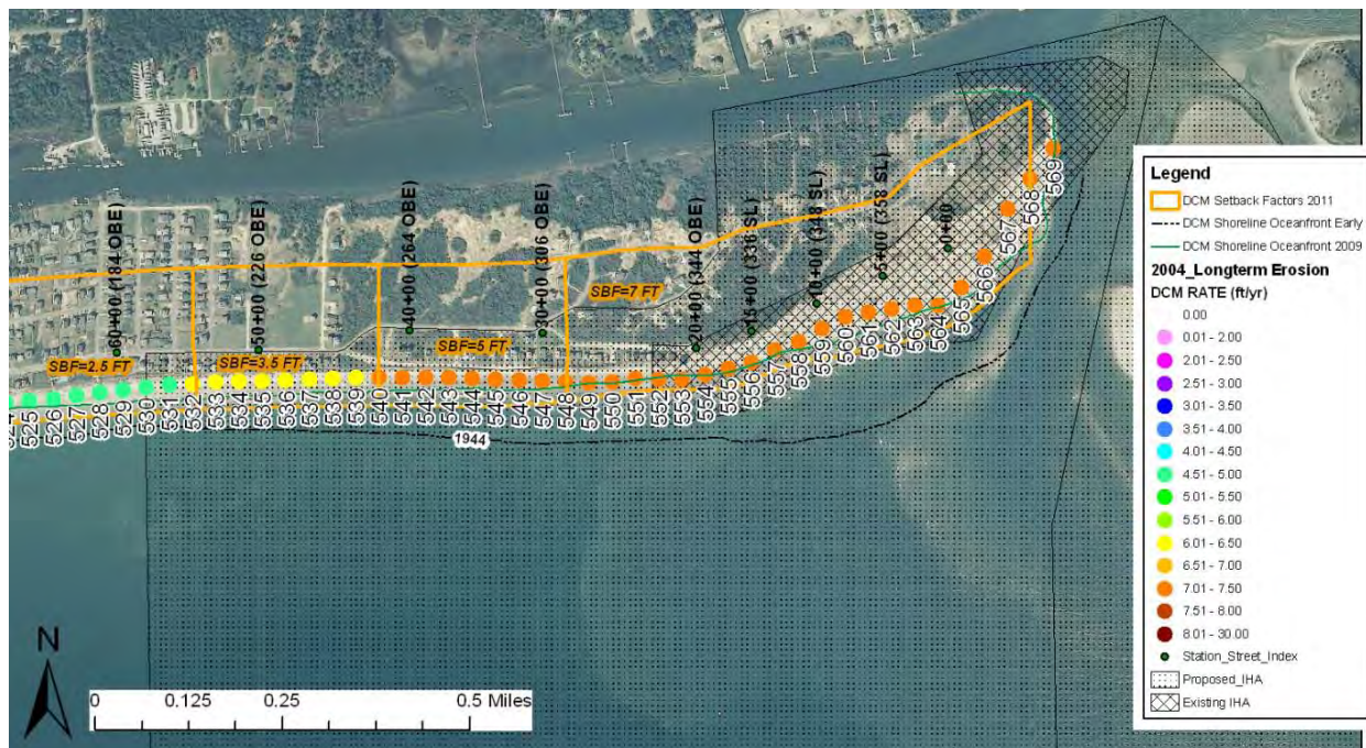
Figure D-6. Current and Proposed IHA Boundaries. 2011 setback factors (SBF) and 2004 erosion rates also pictured.
