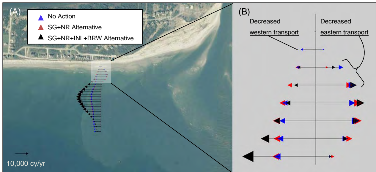
Figure 7-16. (A) HB East Transect Sediment Transport (2004 simulation). (B) Close-Up of Area Affected by Groin. Note decreased eastern (into inlet) and western sediment transport with groin alternatives. Increases in outer transport vectors with groin alternatives can be attributed to increased available sediment from nourishments and the relocated inlet channel.
