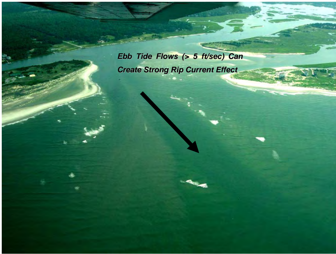
Figure 8-8. Existing Potential for Rip Current Effects at LWF Inlet (8/2005 photo) Source: USACE.
