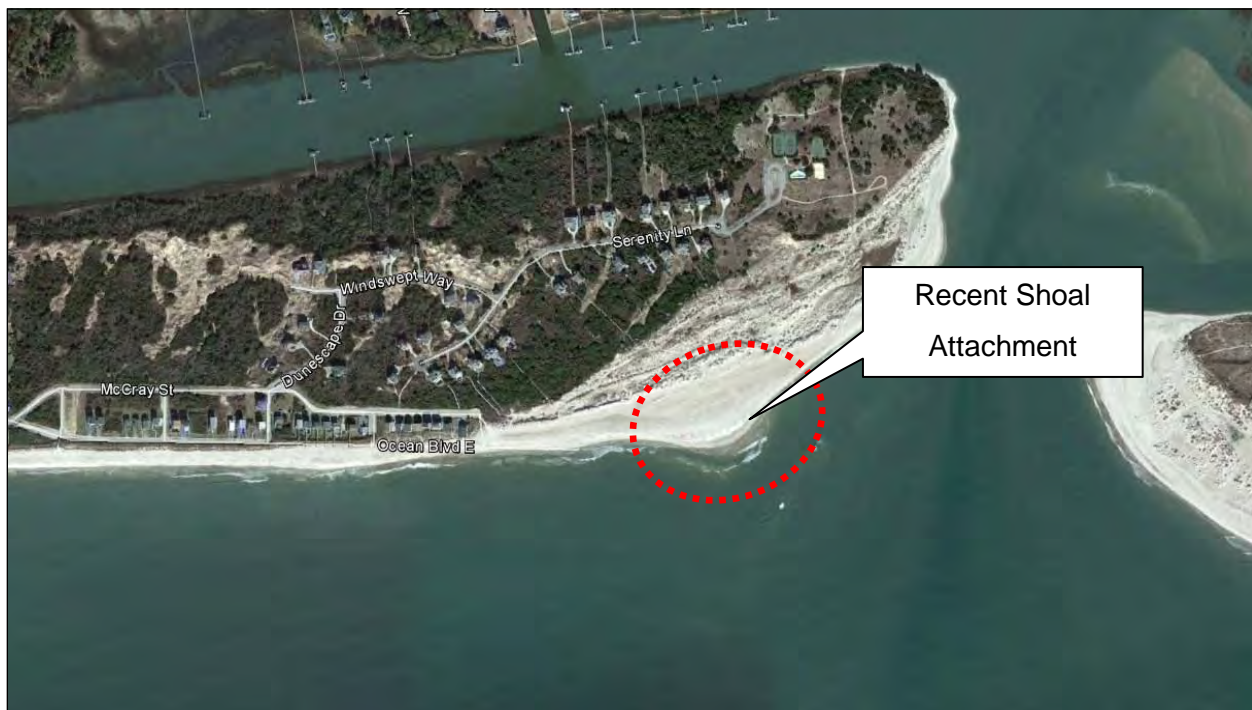
Figure 7-39a. Google Earth Aerial Image from 1/3/2013. Note “bump” in shoreline indicating a recent shoal attachment on the east end (~Station 10+00).
