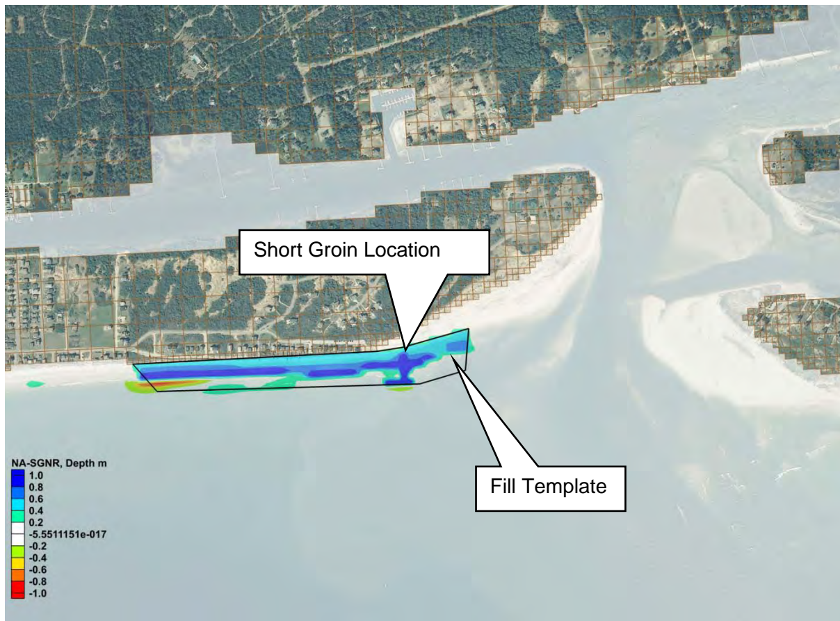
Figure 7-21. One-Year Morphological Differences between the No-Action (NA) and Short Groin and Nourishment (SGNR) Cases. Blue=accretion, red=erosion.
