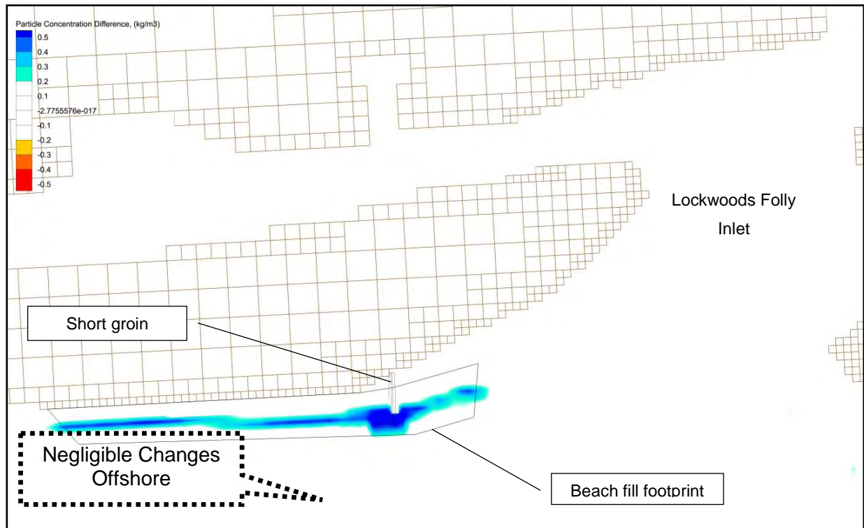
Figure 7-56. Particle Concentration Comparison of No-Action and Short Groin/Nourishment Alternative. Blue indicates the no-action alternative exhibits increased particle concentrations. Significant changes are localized to the nourishment footprint.
