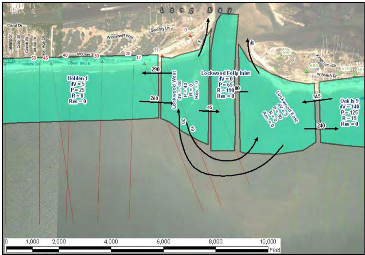
Figure D-14. LWF Inlet sediment budget as developed by OCTI (2008). All values are 1,000 cubic yards (cy) (e.g., 290=290,000 cy). Black arrows indicate sediment transport in/out of cells. dV =annual volume change, P =annual placement, R =annual removal, Res =annual residual.
