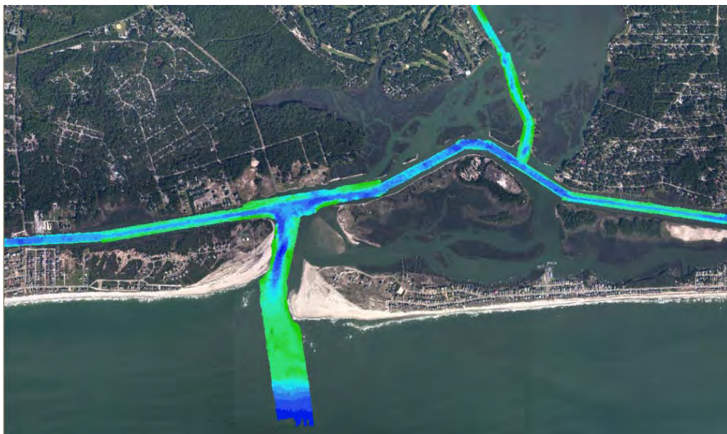
Figure 7-4. Example of USACE Survey Data Coverages (Inlet, AIWW, and LWF River data sets shown).
