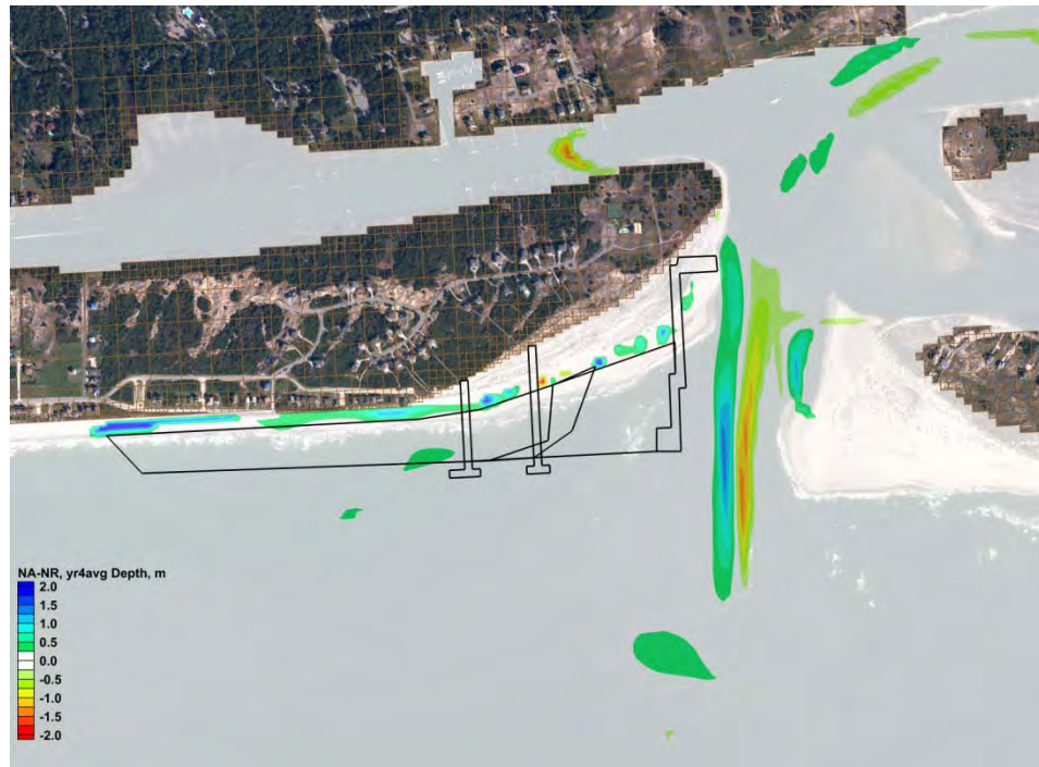
Figure 7-40. Nourishment-Only (NR) Year 4 Average Depths Relative to No-Action (NA). Essentially all nourishment sand has eroded away. Fill and groin templates shown for reference.
