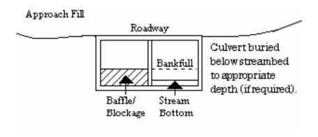
(7) Where adjacent floodplain is available, flows exceeding bankfull will be accommodated by installing culverts/pipes at the floodplain elevation. When multiple culverts/pipes are used, baseflow must be maintained at the appropriate width and depth by the construction of floodplain benches, sills, and/or construction methods to ensure that the overflow culvert(s)/pipe(s) is elevated above the baseflow culvert(s)/pipe(s).
