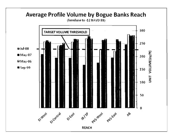
**Fig. 2** – Average profile volumes for September 1999, May 2006, May 2007, and July 2008 for seven oceanfront reaches along Bogue Banks. A target volume threshold of 225 cubic yards per linear foot (cy/ft) was established in 1999 as a benchmark for beach health.
