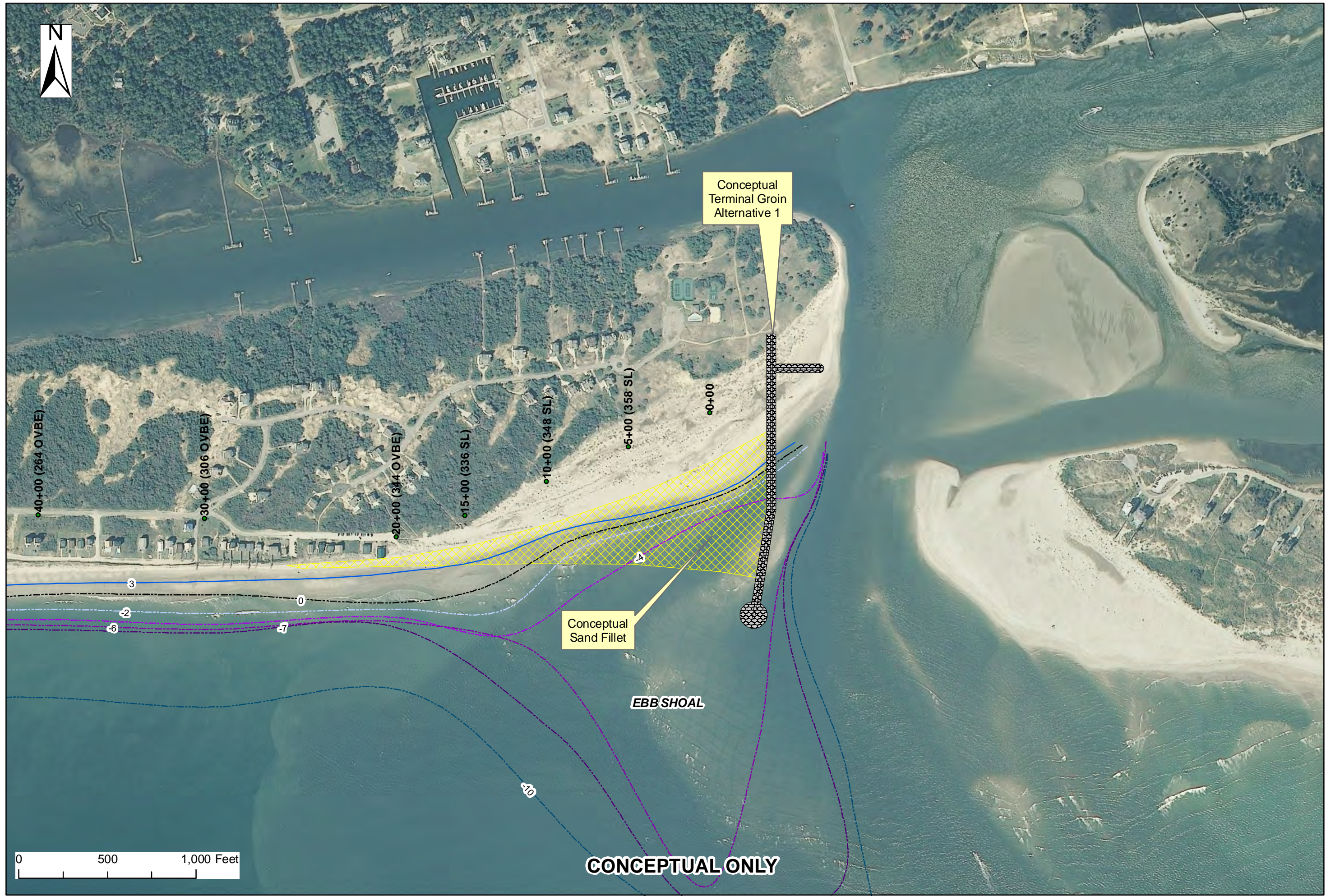
FIGURE 7-1: Conceptual Terminal Groin Alternative 1 East End, Holden Beach 2010 Depth Contours in feet NGVD (MHW=3 ft, MLW=-2 ft); 2008 Aerial
