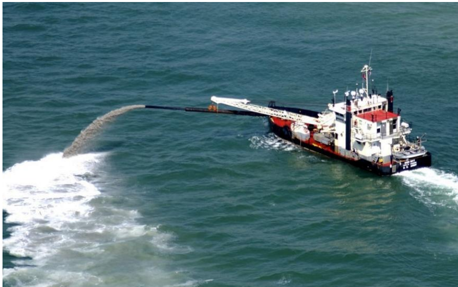
Photo 3.3. Bogue Inlet navigation channel sidecast dredging.
