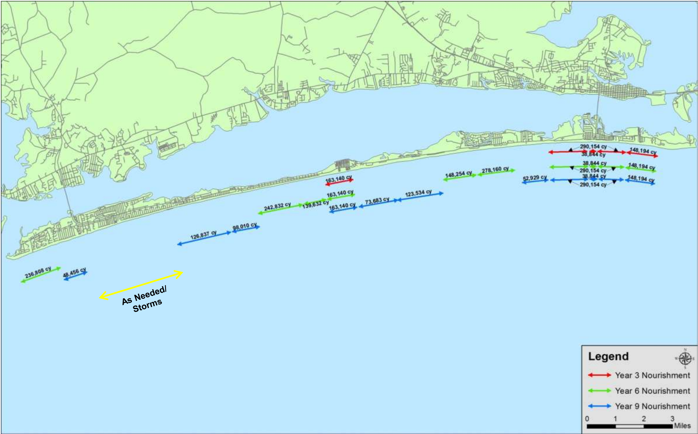
Figure 8-23: Detailed Subreach Nourishment Plan
