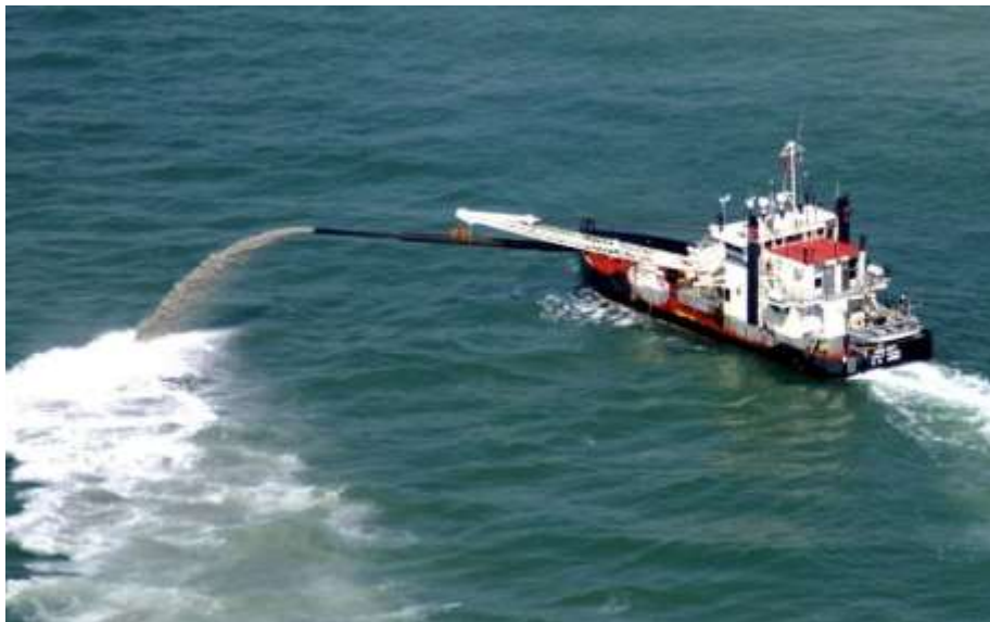
Photo 3.3. Bogue Inlet navigation channel sidecast dredging.
