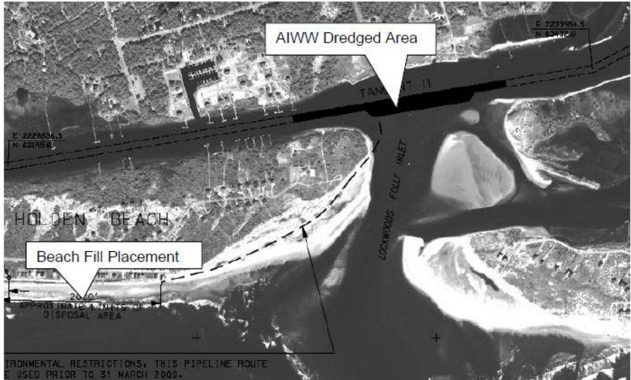
Figure 3.1. USACE LFIX AIWW Dredging and Beach Placement Schematic.
