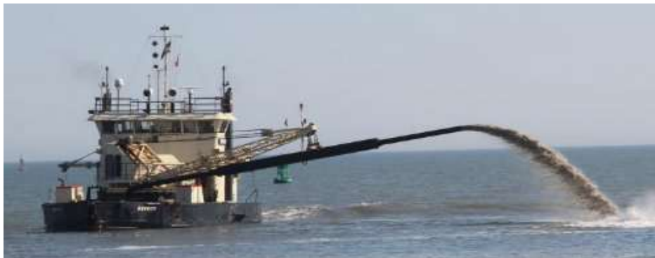
Photo 3.3. View of sidecast dredge, the Merritt, working within the outer bar channel of LFI.
