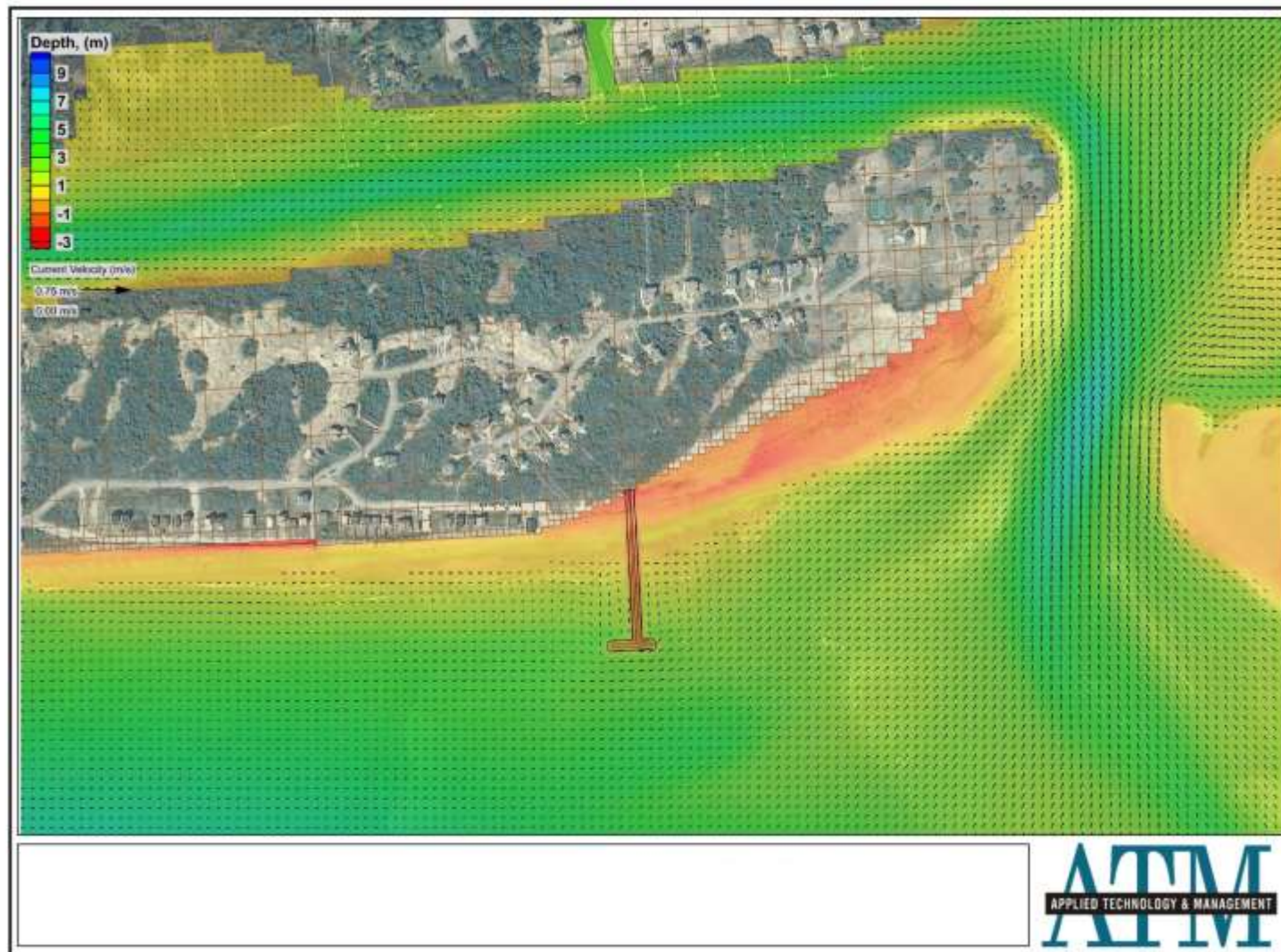
Figure 5.19. Alternative 5 - Typical Flood Tide Current Vector Diagram
