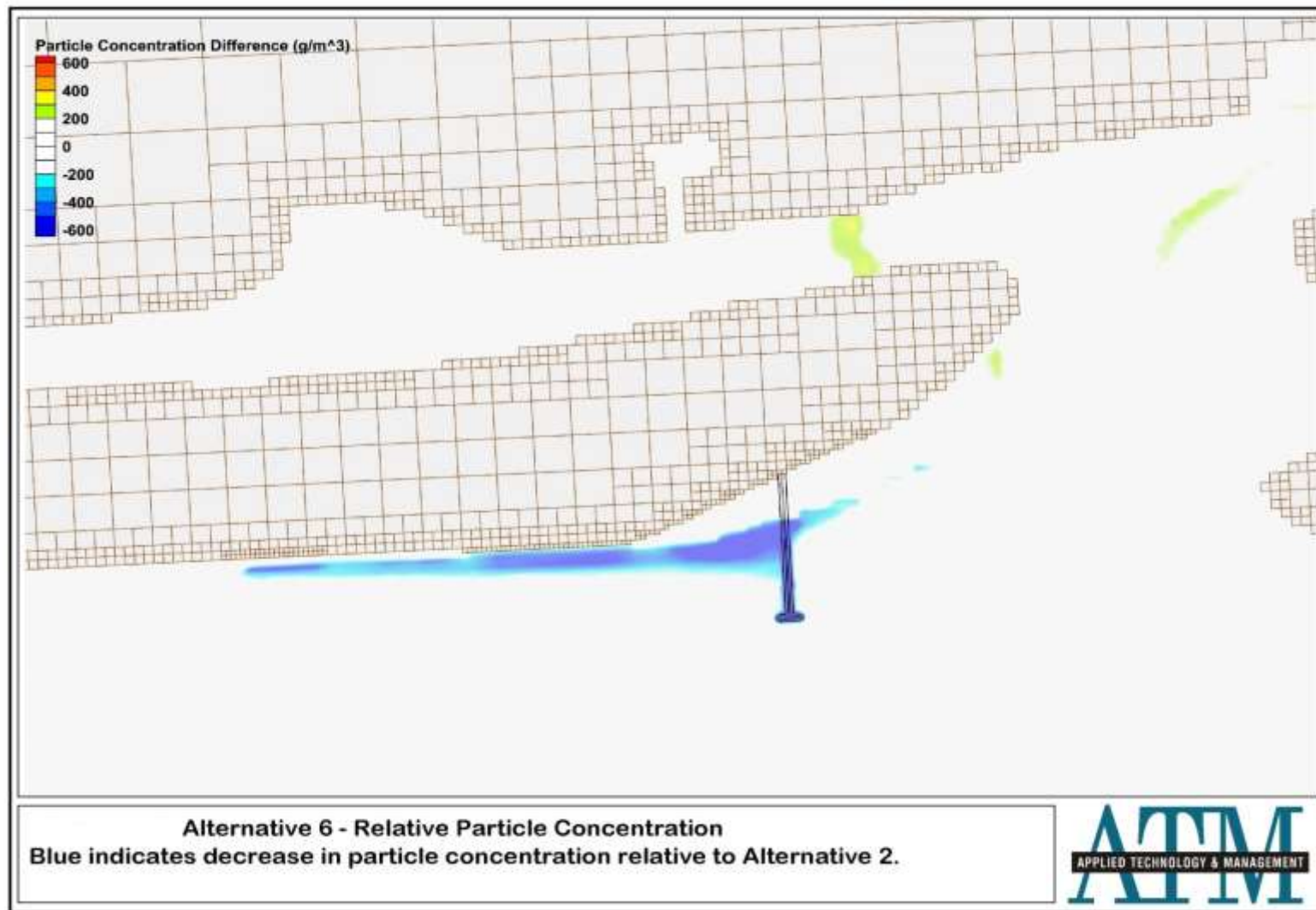
Figure 5.26. Alternative 6 - Relative Particle Concentration
