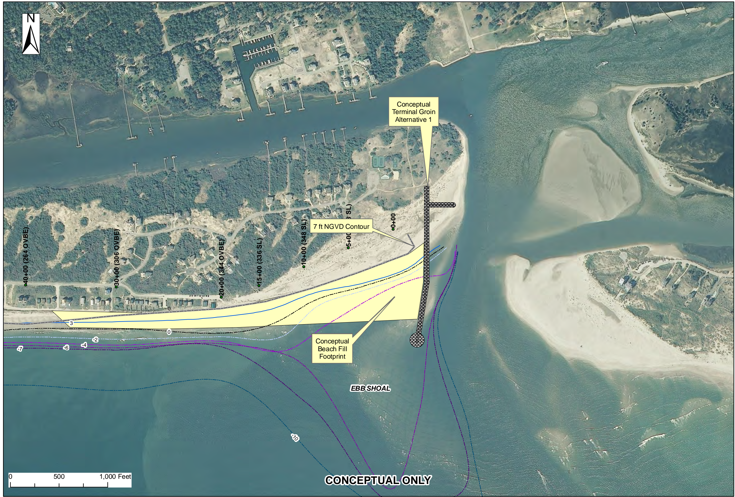
FIGURE 7-5: Conceptual Terminal Groin Alternative 1 with Beach Fill Footprint East End, Holden Beach 2010 Depth Contours in feet NGVD (MHW=3 ft, MLW=-2 ft); 2008 Aerial
