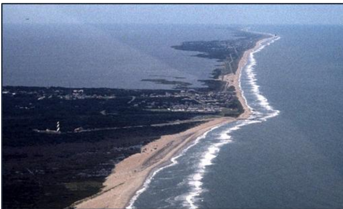
FIGURE 8.4. Oblique aerial photograph looking north of the shoreline “salient” (bulge) produced by three groins fronting the former US Naval Facility and old Cape Hatteras Lighthouse location. [Image courtesy of USACE–Wilmington District taken on 9 September 2000]
