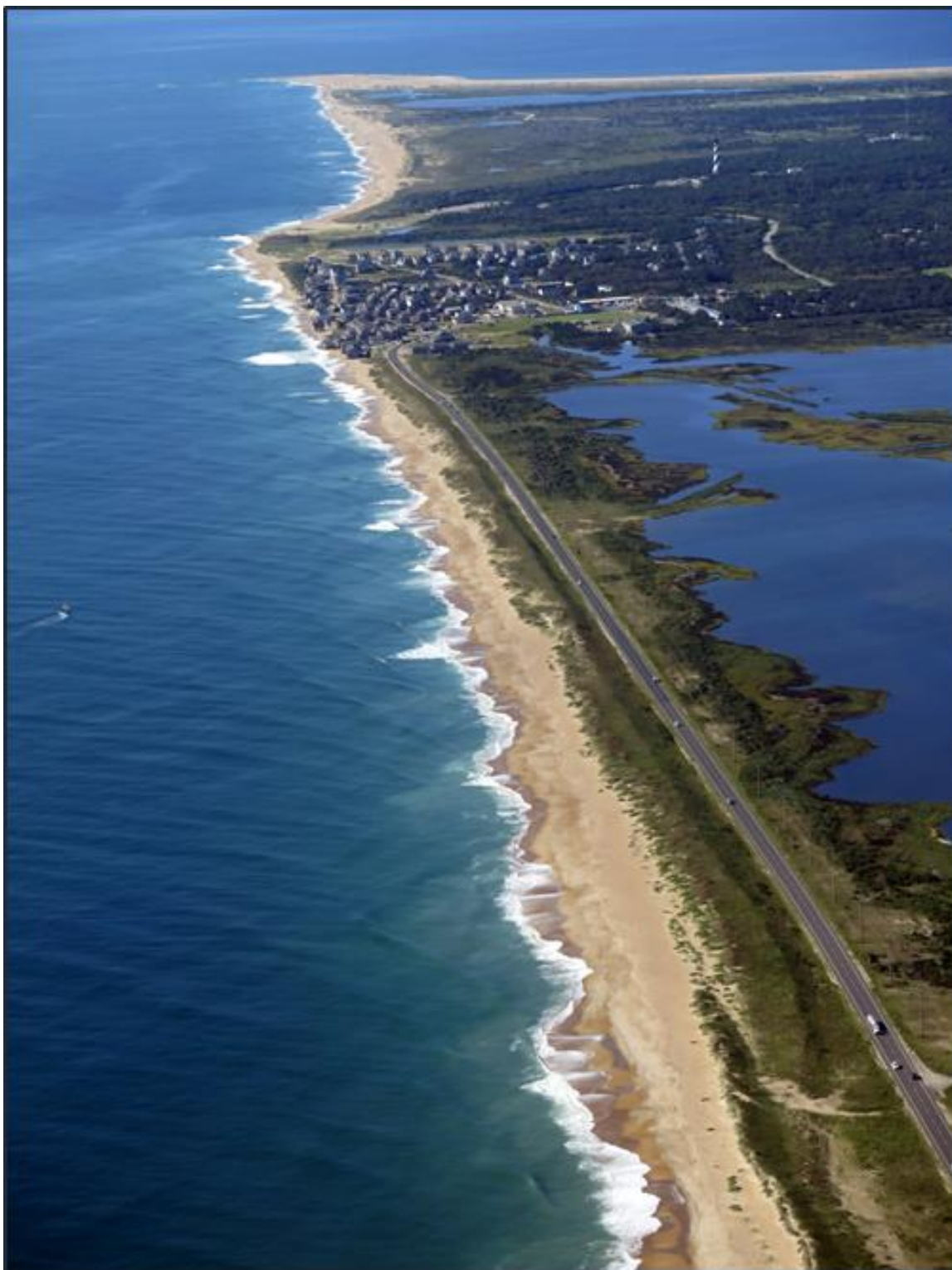
FIGURE 8.6. Project area on 11 September 2014 looking south. The “salient” (bulge) in the shoreline is situated at the south end of Buxton Village at the former site of Cape Hatteras Lighthouse and three groins which were constructed in 1970 by the US Navy. [Image by CSE]
