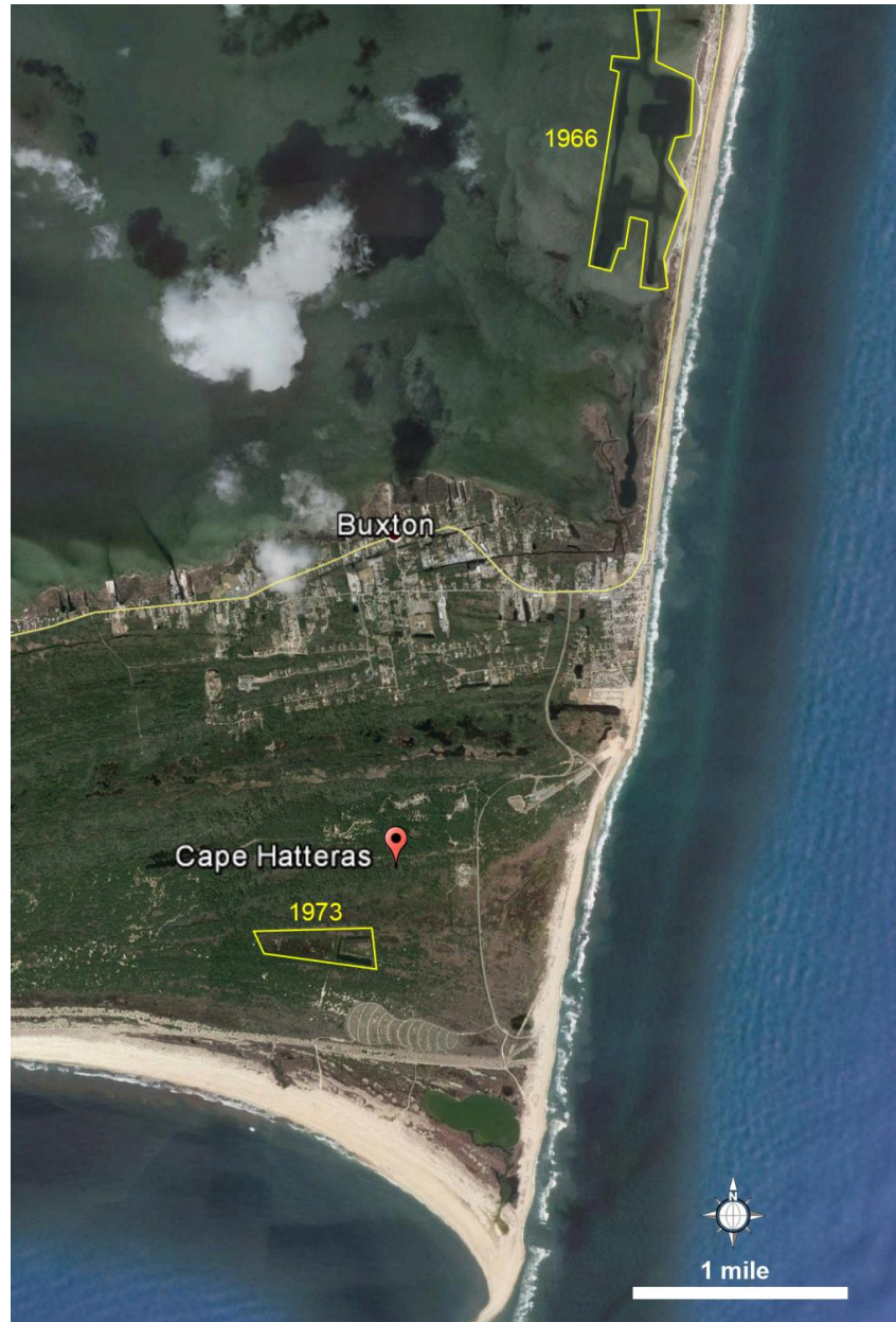
FIGURE 8.1. Aerial image of the project area in January 2014 showing relict borrow areas in Pamlico Sound likely used in a 1966 beach nourishment project (source: Google Earth). An inland pit within the Cape Point area of Seashore was excavated and used for borrow material during the 1971 and 1973 nourishment projects.
