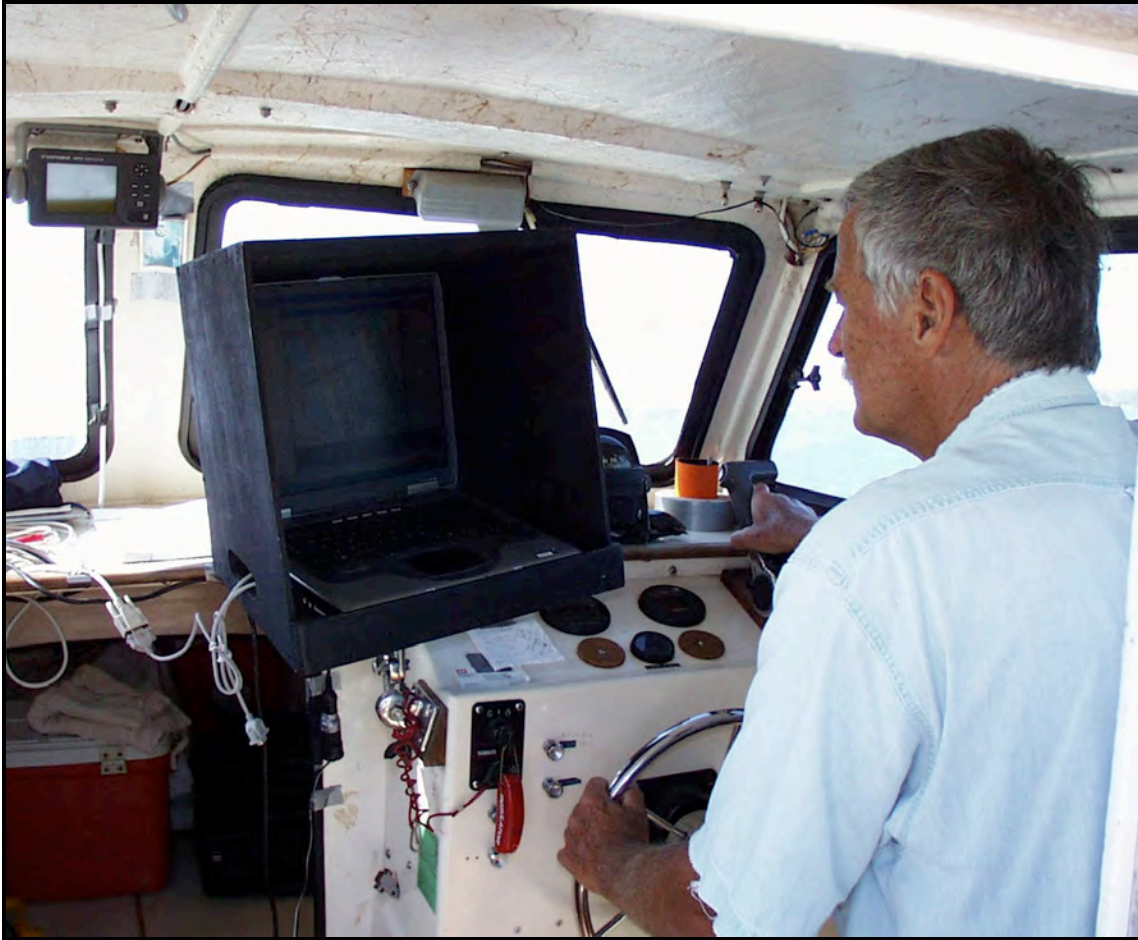
Figure 8. Monitoring computer navigation system located at vessel helm.
