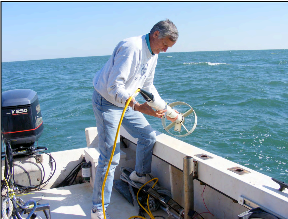
Figure 5. Deploying EG&G GEOMETRICS G-881 cesium vapor magnetometer.
