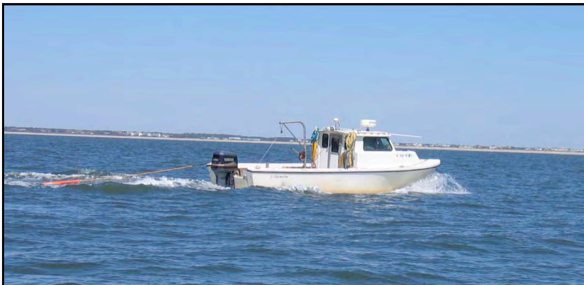
Figure 4. Twenty-five foot Parker survey vessel, the Tidewater Surveyor .
