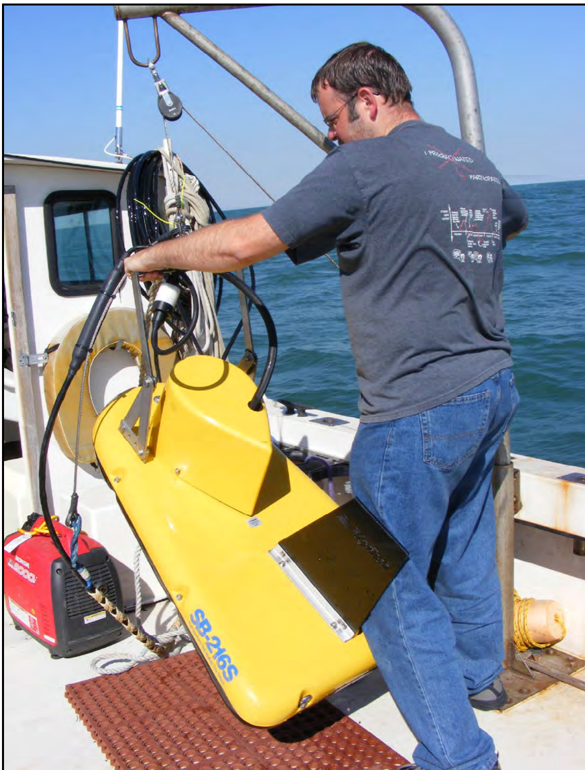
Figure 7. Deploying the EDGETECH sub-bottom 216S tow vehicle.
