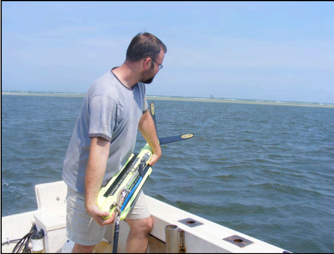
Figure 6. Deploying the KLEIN 3900 digital sidescan sonar.
