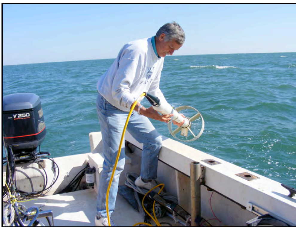
Figure 3. The EG&G GEOMETRICS G-881 cesium vapor magnetometer.
