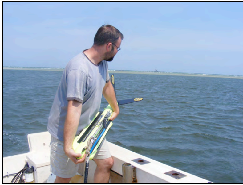
Figure 4. The KLEIN SYSTEM 3900 digital sidescan sonar.
