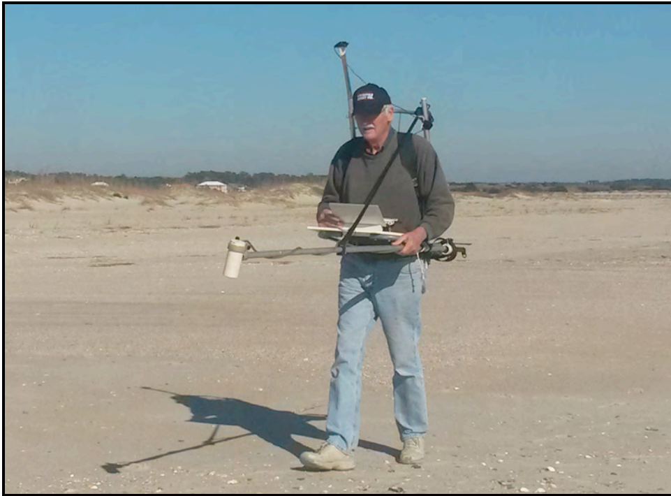
Figure 6. The Geometrics G-856 magnetometer and Trimble DGPS terrestrial survey.
