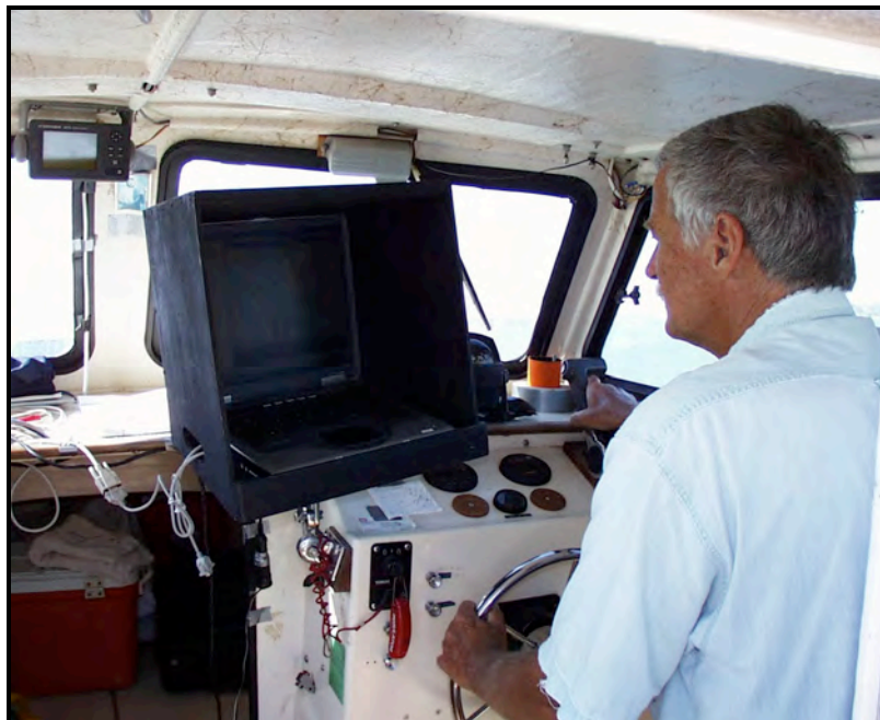
Figure 5. Computer navigation system located on the research vessel helm.
