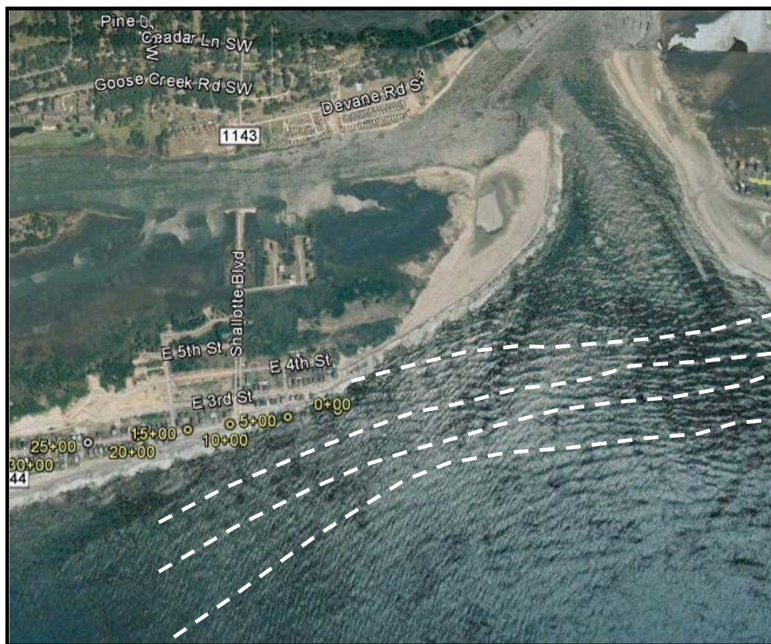
Figure 5.8. Wave refraction at Shallotte Inlet, October 2009.
